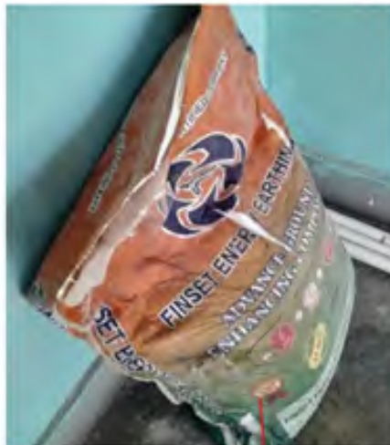
Earthing Chemical (Bentonite /Graphite)
